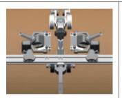
Work with 2 PA probes for PA testing on pipe with diameter large than 100mm.
