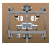
Work with 2 PA probes and 1 pair of TOFD probes for PA and TOFD testing on pipe with diameter large than 300mm.
