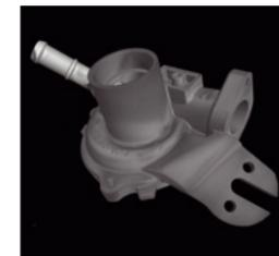
Turbocharger cast housing
